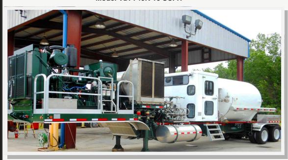
Self-contained liquid nitrogen pumping and vaporization system equipped with (17) Million BTU/h fired vaporizer, capable of flow rates up to 740,000 SCFH and working pressures up to 10,000 psi. The unit is designed efficiently to perform well servicing, industrial and pipeline applications. The trailer-mounted system conforms to US DOT regulations in terms of weight distribution, roading dimensions, and cryogenic tank construction.
